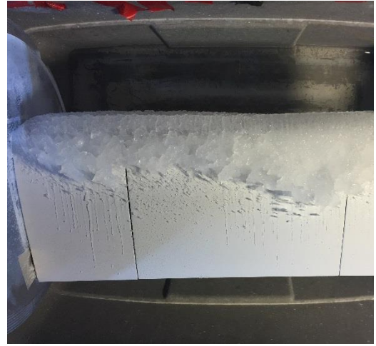
Final ice accretion shape on the model (Pressure surface) (Coating-A2, V_{\infty}=40 m/s, LWC=2 g/m 3 , T=-8^{\circ}\text{C} , \alpha=-5^{\circ} )
